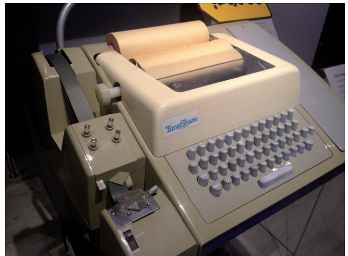
Figure 2: Typical teletypewriter as used in the early days of interactive computing [i]
