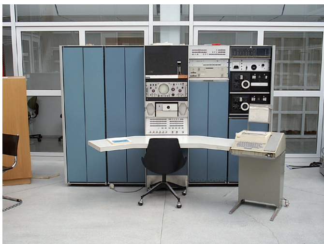
Figure 4: DEC PDP-7 – the first UNICS created by Ken Thompson and Dennis Ritchie ran on a PDP-7 [iii]
