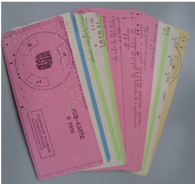
Figure 1: Punch card stack including control cards, FORTRAN source code cards and data cards
